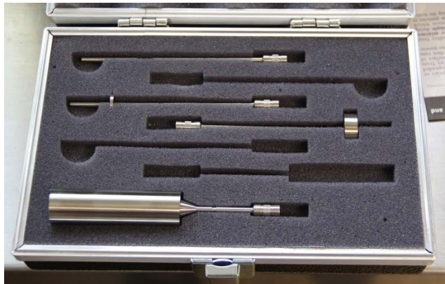
Figure 2: Brookfield DV2T-LV Viscometer spindle selection. Lightest viscosity range on the bottom going to heaviest at the top.
