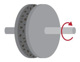
Contaminats in barrier fluids can increase seal wear. SLFi barrier fluids are manufactured to meet ISO Cleanliness Code of 8/5
